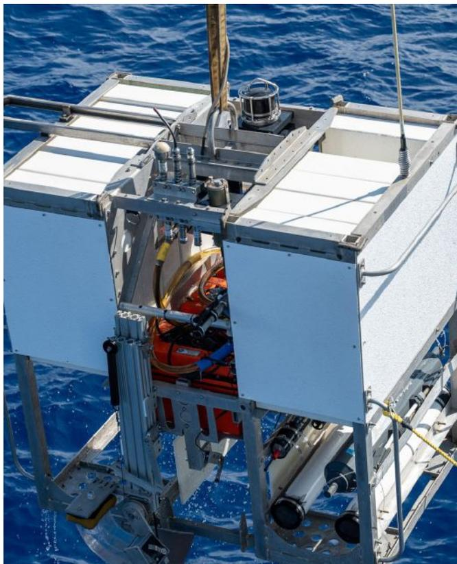
Figure 2: Deep dive of the new AquapHOx deep sea logger with the new optical pH sensor for the total scale in the Hawaiian Islands. (Credit: Discover Our Oceans LLC)
