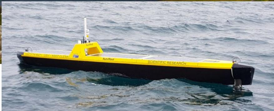
Given the challenges we face with a changing climate, developing long-endurance, net-zero capability in ocean observations have never been more important. As well as meeting low-emission requirements, the modest speed and sound of the wave propelled AutoNaut uncrewed surface vessel (USV) is proving an asset in detecting marine mammals. The vocalizations of whales and dolphins were recently recorded throughout two passive acoustic baseline surveys in West Africa and Scotland.
